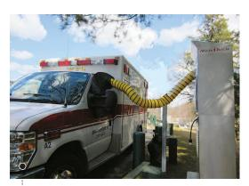
BREATHE EASY The MediDock idle-elimination system is a full-service docking station for ambulances that provides stationary power for on-board batteries and medical equipment plus HVAC for temperature control inside the vehicle. Ambulance drivers can shut off their engines without fear of losing power to the batteries and any medical equipment that needs to be regulated at specific temperatures.
