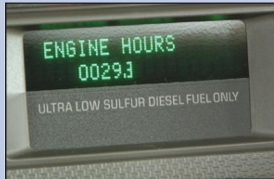
In addition to oil, oil filter & fuel filter maintenance, the engine coolant system nitrite level should be checked at the mileage or equivalent hour intervals specified by the maintenance schedule. For example, when operating the 2009 Super Duty 6.4L Power Stroke® diesel engine equipped truck under Special Operating Conditions, coolant nitrite level should be checked every 20,000 miles or 800 hours of operation.
